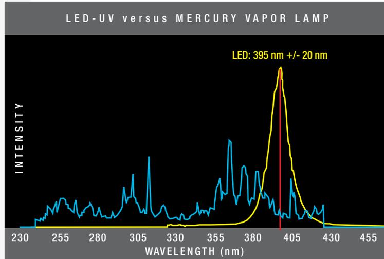
*By operating at very specific wavelengths, LED lamps have the potential to be much more efficient than their broad-spectrum mercury counterparts. These narrow wavelengths mean that LED lights are far more selective in the photoinitiators they trigger.*
