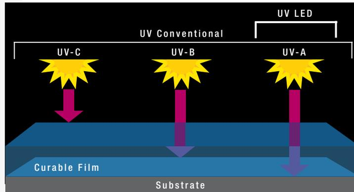
*How different UV light penetrates materials depends on the wavelength generated. By carefully matching the photoinitiator and light source, it is possible to simultaneously achieve both surface and deep section curing.*
