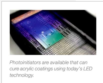
*Photoinitiators are available that can cure acrylic coatings using today's LED technology.*
