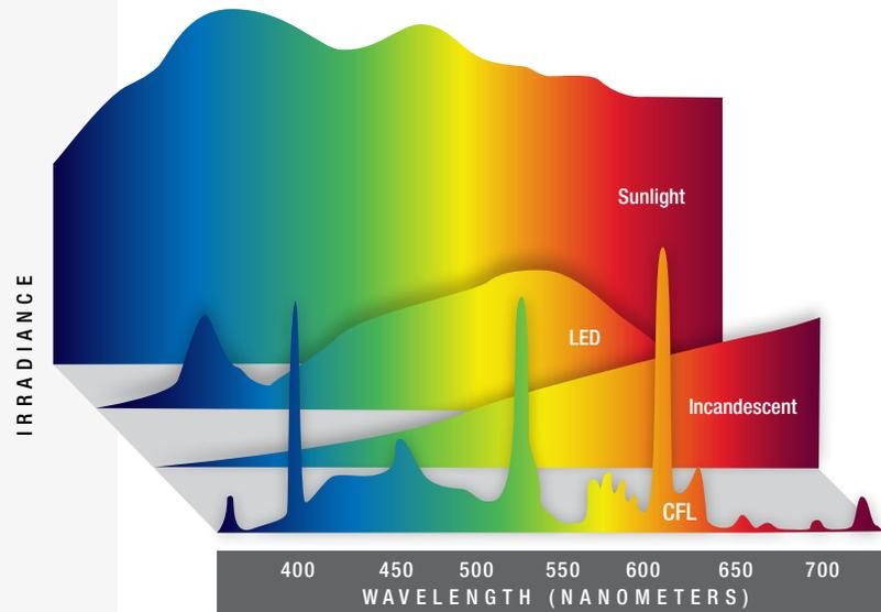
*Light sources emit energy at different wavelengths, as shown above. Although the human eye cannot discern these individual wavelengths, the photoinitiators that operate in UV cured materials are highly specific in the wavelength(s) that activate them. Make sure your UV light source has the output wavelength required by your photoinitiator.*
