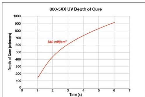
Product was UV cured using an F300S/F300SQ Fusion UV System equipped with a standard "H" bulb.
