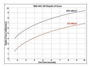
Product was UV cured using an F300S/F300SQ Fusion UV System equipped with a standard "H" bulb.
