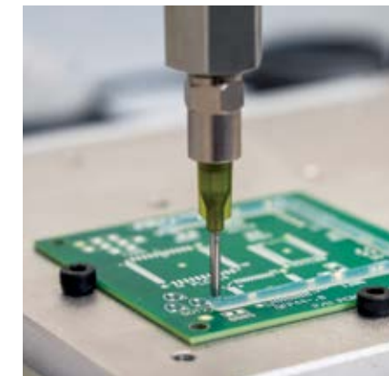
800-400 applied as part of a dam and fill process.
