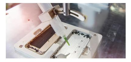
Novagard 500 Series Electronic Silicones with low/medium viscosity are conformal coatings. They are preferable to paste-consistency products where flow coating is the preferred application method and when flow into small crevices and hard to reach places is desired.
